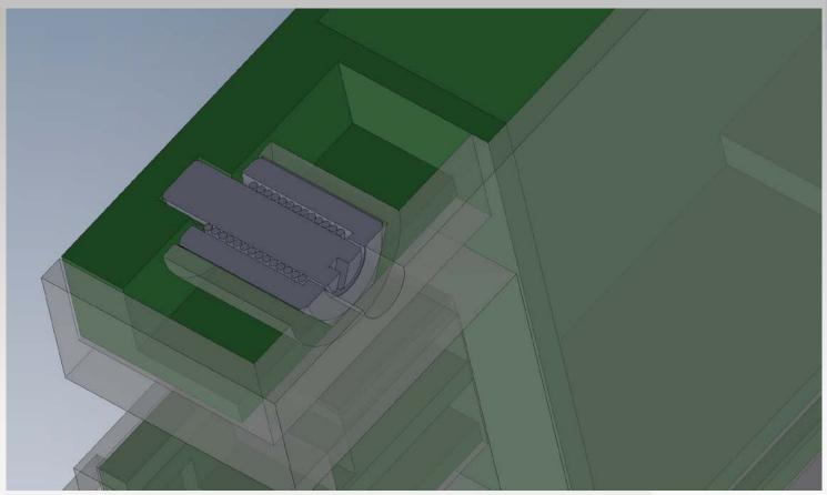
Only the screw head is seen from the unlawful access person and the internal mechanism is not understood. Therefore, when the screw runs idle, it misunderstands it.
