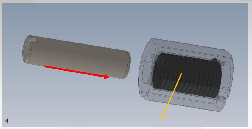
The stick to recognize the dummy screw doesn't turn in the opposite direction though it turns in the direction of a positive rotation of the screw tightening by spring in the housing.
